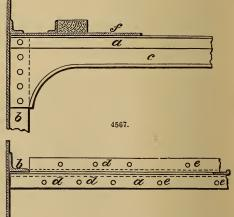
The holes for riveting stringer-plate to angle-iron on beams should be about eight times the diameter of the rivets apart.
